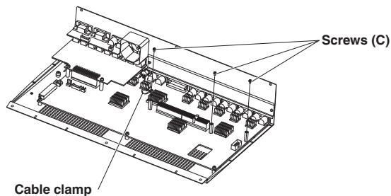
⑥ Insert the HD analog board from the inside of the rear panel, and insert it along the guide rail for the connector. (Insert it securely and completely.)
