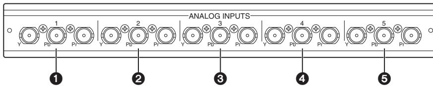
**① to ⑤: Analog HD component input connectors [ANALOG INPUTS 1 to 5]**
